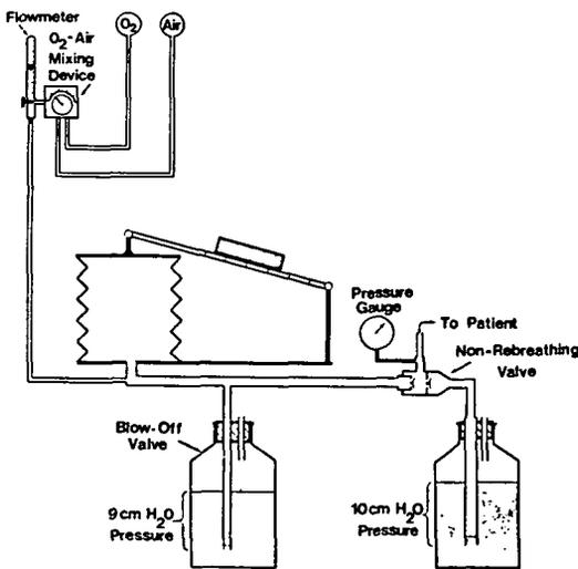
FIG. 1. CPAP circuit using weighted bellows.
