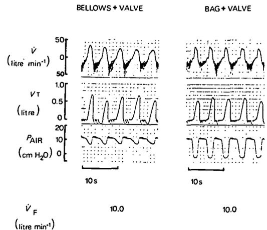
FIG. 2. Comparison of flow ( $\dot{V}$ ), tidal volume ( $V_T$ ) and airway pressure ( $P_{AIR}$ ) recorded at the mouth at a fresh flow rate ( $\dot{V}_F$ ) of 10 litre min<sup>-1</sup> using the bellows and the bag CPAP systems.
