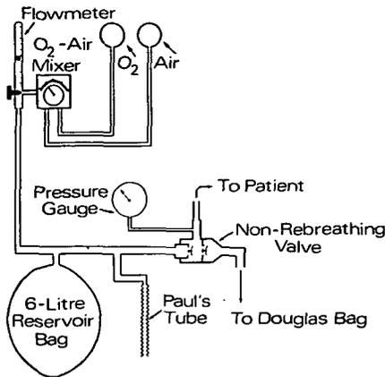
FIG. 3. The system for spontaneous breathing at ambient pressure. The Paul's drainage tube acts as a low resistance non-return valve and prevents overflow through the inspiratory and expiratory flaps of the non-rebreathing valve.
